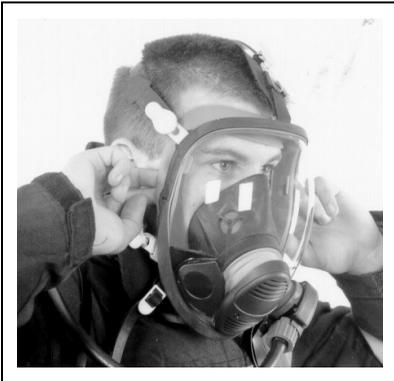
With the cylinder valve open, insert a finger under faceseal and check for a steady outward flow of air. Remove finger and allow mask to re-seal.
