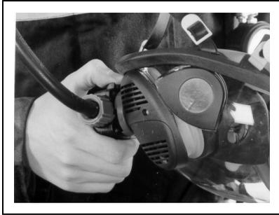
3. Check that the flat on the DV bypass knob is off (flat on the knob is towards the facemask).
