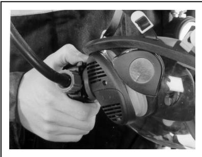
1. Fit the DV of a breathing or airline apparatus, for which **VISION 3** is approved, to the facemask.
