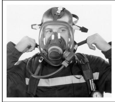
2. Adjust the facemask top strap so that the mask is at the correct level with the face and the head-harness pad is in the centre of the back of the head, then tighten harness straps in sequence: **Bottom, Middle, Top**. DO NOT over-tighten.
