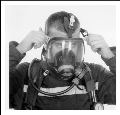
2. Release the head-harness by pulling the harness buckles forwards. Remove mask and let it hang from the neck-strap.
