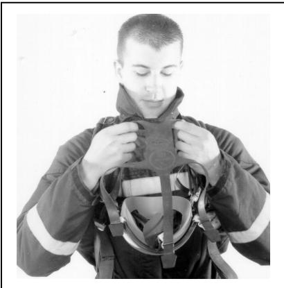
1. Hold the head-harness lower straps, place chin in chin-cup and pull straps over back of head, brushing hair away from face seal.
