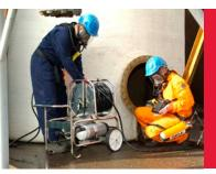
Ideal for environments where ambient oxygen cannot be guaranteed, airline breathing apparatus combines the highest degree of respiratory protection with long duration use.
